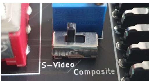
On the V5 and V5.1 versions of the Commodore 128 40/80 Column Video Adapter a secondary switch is added. This switch lets you select the output for the 40 column display. Either Composite (CVBS) or SVideo - Luma/Chroma (Y/C). Best results are generally achieved in SVideo mode. But if you use a third party Scart - HDMI converter, the result is depending on the quality of the converter. Results may vary.
